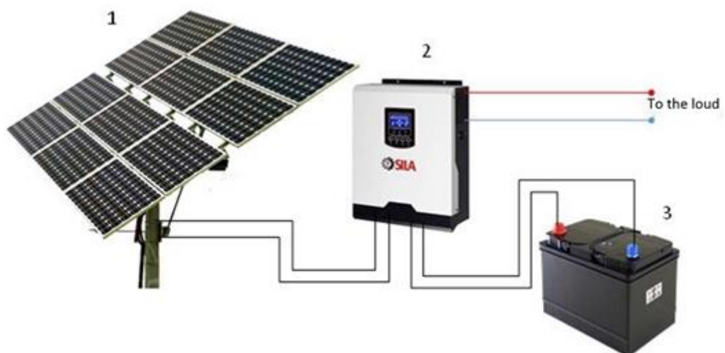
Figure 1.2 - Composition of the PVS: 1 - Solar battery, 2 - battery charge controller and inverter in one case, 3 - battery
